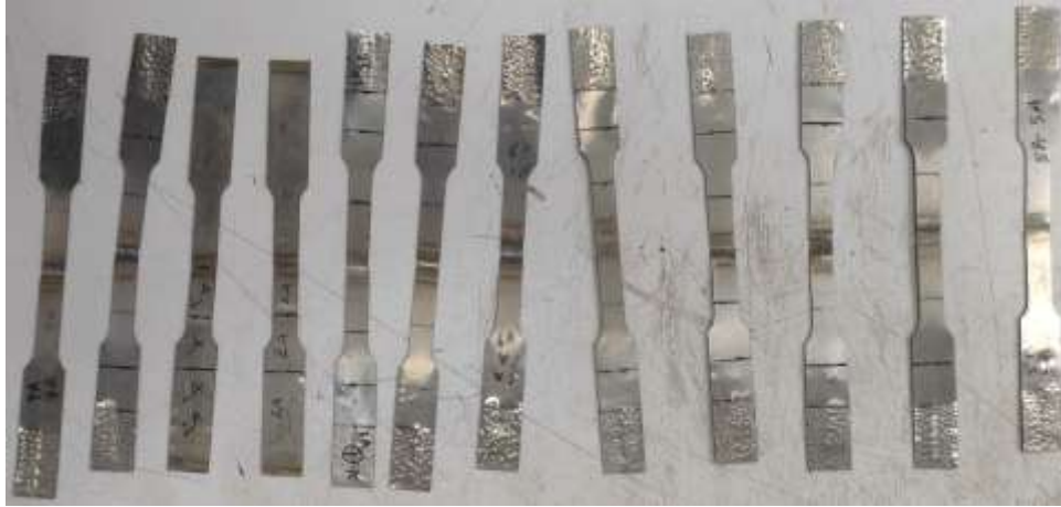
Figure 3 : Some tensile test specimens.
