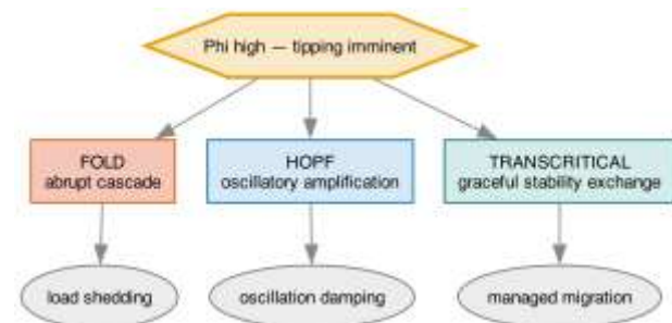
Fig. 2. Bifurcation regimes and matched interventions (illustrative). A fold drives an abrupt cascade (load shedding), a Hopf bifurcation drives oscillatory amplification (damping), and a transcritical transition is a graceful stability exchange (managed migration).
