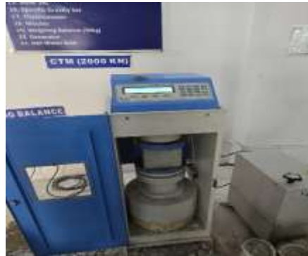
Figure 4.1 Compressive Strength Test
