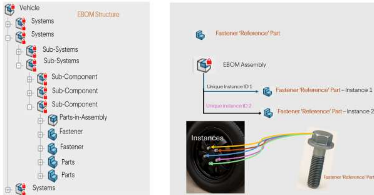
FIGURE 2. Image showing EBOM structure and difference in reference vs instance.
