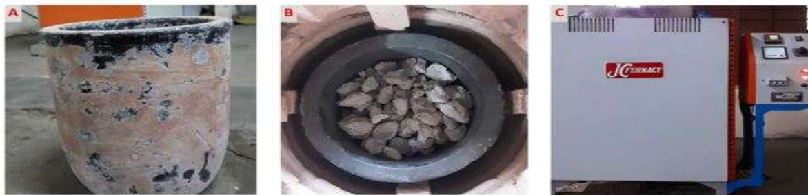
Figure 3.2: (a) A crucible weighing 5 kg was used in the pit furnace. (b) The crucible was filled with 5 kg of concrete waste. (c) The pit furnace heated the concrete waste to 500°C.
