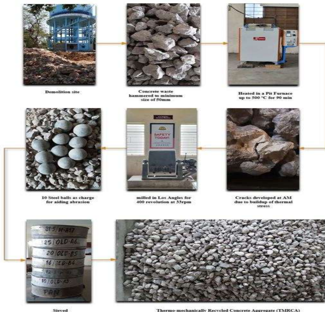
Figure 3.3 Schematic of the methodology adopted for extracting TMRCA from waste chunks
